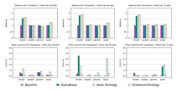
Figure 7: Speed-up and power cap error with transactions
