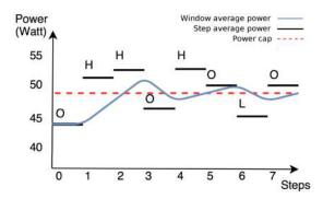
Figure 5: Example of fluctuations of configurations performed by the enhanced strategy in-between different exploration procedures. Window size is set to 8. O denotes the configuration  $(p,t)^*$ , H the configuration  $(p,t)^H$  and L the configuration  $(p,t)^L$ . These configurations are fixed along each window but their power consumption could change.
