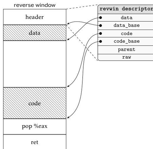
**Figure 3.4.** The figure illustrates the structure of a single reverse window, binding its descriptor's fields described in Table 3.1 to the actual representation in memory. Note that the reverse-window descriptor's raw field references a bare memory area where to store both code and data. At the same time, the window's descriptor is contained into the same memory area as an header.
