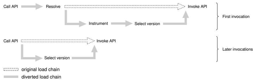
**Figure 5.2.** High-level dynamic symbol's address resolution flow for the shared objects.
