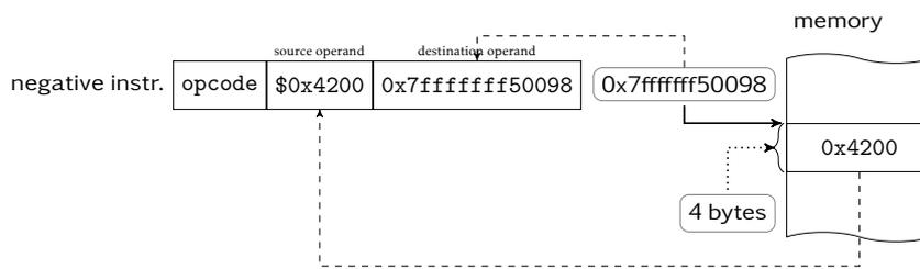
**Figure 3.9.** The engine creates an inverse instruction encoding in the instruction’s binary representation the destination address as a destination operand and the current value of that memory location as the source operand. The amount of bytes to be read for this task depends on the argument of the engine’s invocation.
