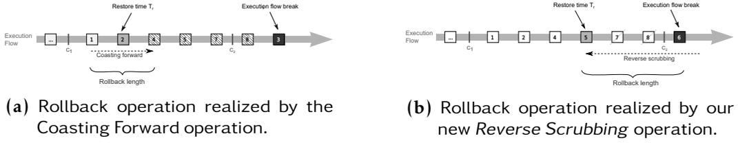
**Figure 4.2.** According to the relative distance of the generic checkpoint  $C_x$  to the restoration point  $t_r$ , our hybrid rollback strategy combines the coasting forward operation employed by the conventional state saving strategy (a) and our new *reverse scrubbing* operation exploited by the approach based on reverse windows (b).
