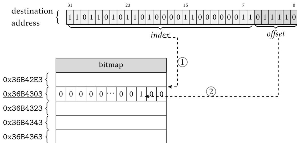
**Figure 3.13.** The index bitmask is used to first compute the family range ① of the destination address; then we harness the offset bitmask to displace within the reverse cache to the related presence bit ②.
