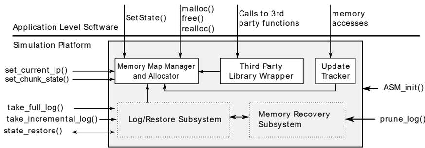
**Figure 4.3.** Architecture of the DyMeLoR memory manager of ROOT-Sim
