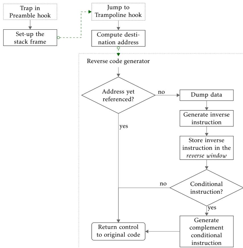
Figure 3.10. Flowchart of our reversal engine.
