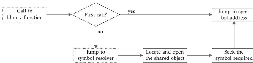
Figure 5.4. Flowchart of the dynamic symbol resolver.
