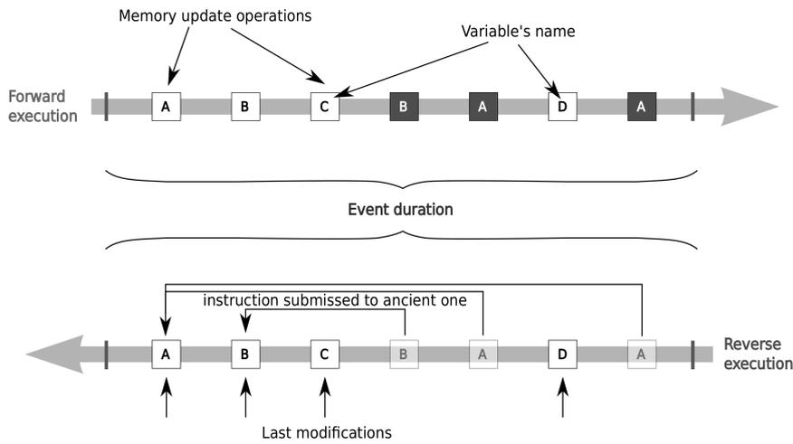
**Figure 3.11.** Illustration of the instruction predominance property. Every address that is previously involved in a negative instruction will be overwritten by the following negative instruction. In fact, the last reverse update on that address would be the one relative to the first reference to that address.
