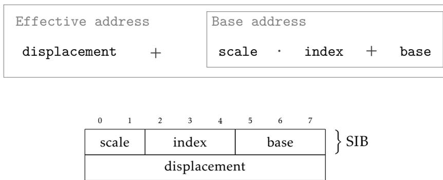
**Figure 3.8.** The x86's complete addressing mode. The SIB byte represents the tuple  $\langle \text{scale}, \text{index}, \text{base} \rangle$ , where parameters *index* and *base* are register's identifiers; we subsume their content, for the sake of brevity. Both *displacement* and *scale* are wired into the instruction encoding.
