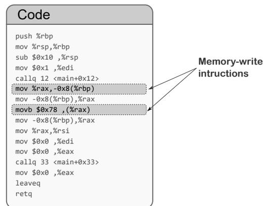
**Figure 3.2.** Example of an assembly program which makes updates on memory.
