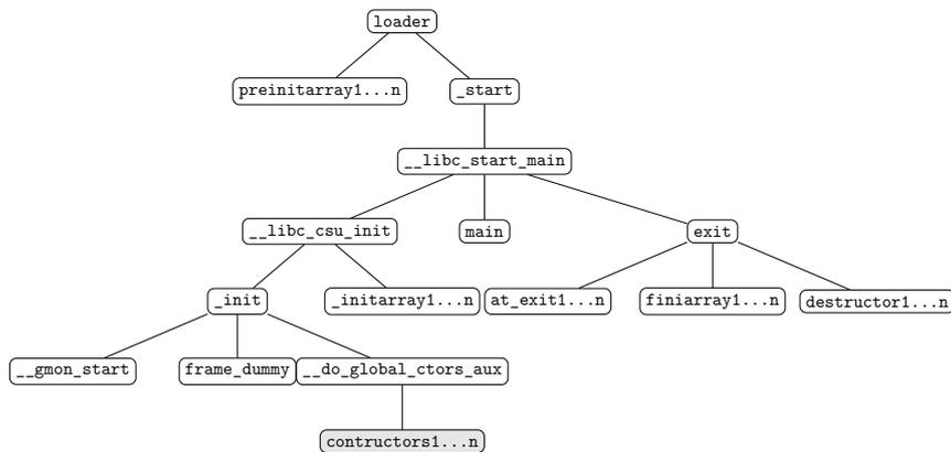
**Figure 5.1.** The whole picture of the functions call chain to start a new process in Unix-like Operating Systems.
