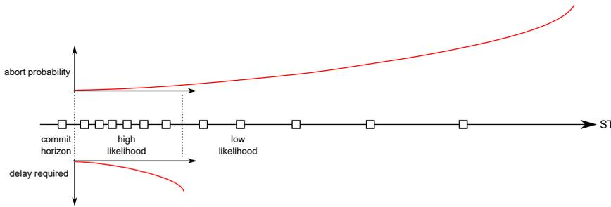
**Figure A.1.** Three logical regions on the simulation time (ST) axis, with varying density of pending events—those still to be processed, which will possibly generate new ones.
