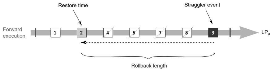
**Figure 4.1.** Basic reverse schema to employ reverse window in a rollback operation.
