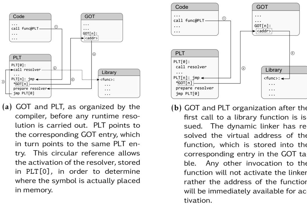
**Figure 5.3.** Dynamic symbols resolution procedure relying on the GOT and PLT tables.
