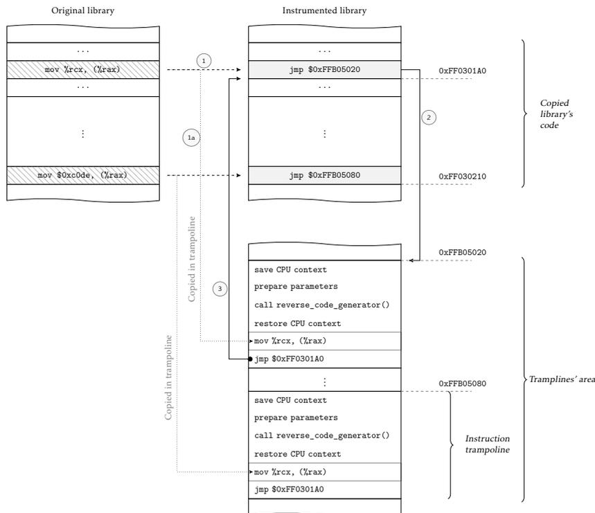
**Figure 5.5.** First the memory-write instruction is replaced by a direct jump to trampoline (1); this jump points to the runtime-generated trampoline snippet that contains the original instruction (1a); the jump points to the trampoline's snippet (2), and finally once generated the inverse instruction trampoline's code return control to next instruction of the library's function (3).
