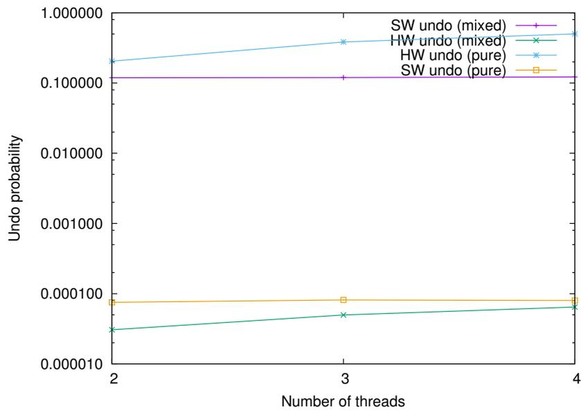
(b) Undo probability for HW and SW speculatively processed events.
