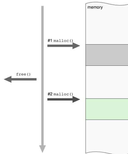
**Figure 3.17.** Subsequent invocations of `malloc` and `free` functions do not ensure the same memory area is reassigned deterministically. The figure illustrates the case of a sequence of `malloc-free-malloc` calls.
