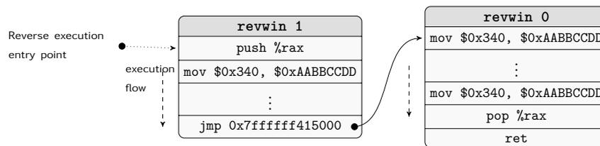
**Figure 3.5.** Chain of reverse windows in case of an overflow of the parent.
