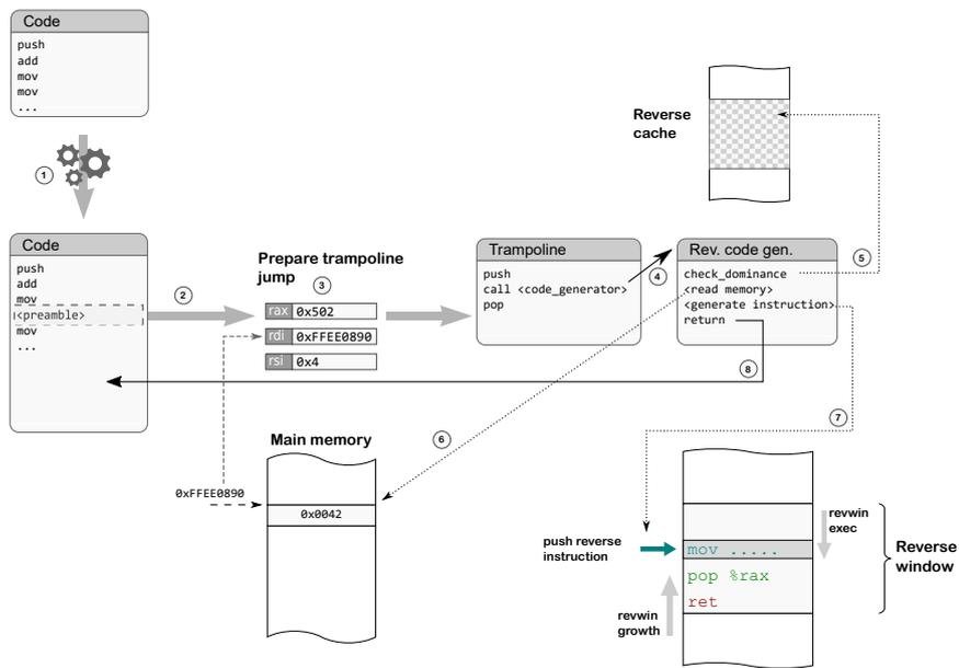
Figure 3.6. The reversing toolchain steps.
