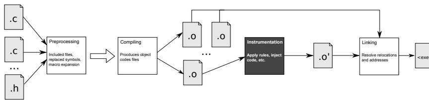
**Figure 3.14.** The Hijacker workflow within the compilation toolchain.
