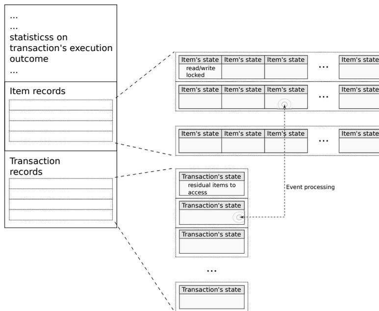
**Figure 4.8.** Layout of the LP state in the data store model.
