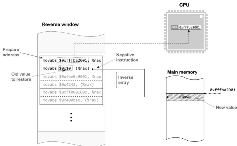
Figure 3.3. Illustration of the content of a single reverse window.
