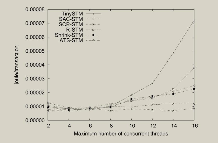
Figure: Per-Transaction Energy Consumption
