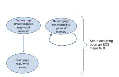
Fig. 3. OS-kernel level page access right manipulation upon an ECS major fault.
