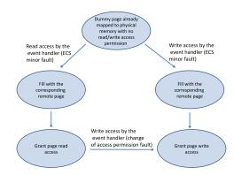
Fig. 4. OS-kernel level evolution of a physicalmemory mapped dummy page within the ECS distributed middleware.
