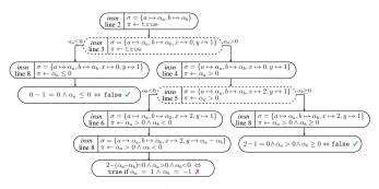
Fig. 3: Execution tree of the example program in Fig. 2. Dashed boxes correspond to states in which a branch is taken. The leave node marked with a  $\times$  is associated with a terminal state which violates the assert () in the example program.
