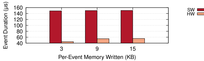
FIGURE 14 Case Study: Event processing duration in an HPC- and software-based incremental checkpointing for speculative simulation.
