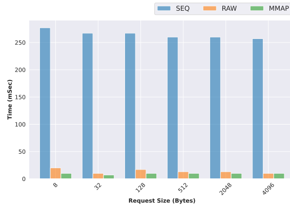
FIGURE 3.12: Time to fully read kernel level data via mmap- and VFS-based solutions.
