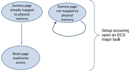
Fig. 3. OS-kernel level page access right manipulation upon an ECS major fault.
