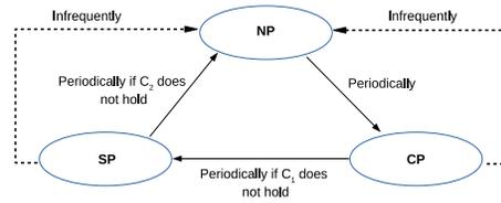
Fig. 6. The state machine driving the selection of prefetch vs non-prefetch policies.
