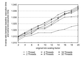
Fig. 5. Extra-tick overhead vs variations of both the extra-tick period and the number of threads.
