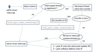
Fig. 16. Behavior of the top-half hook for the LAPIC-timer interrupt.
