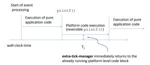
Fig. 4. Management of extra-ticks in the interleave between application and platform code blocks within an event processing wall-clock-time window.
